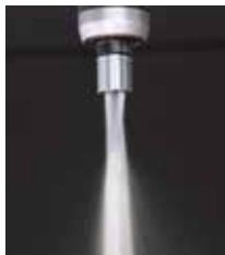
Through tool Coolant is supplied through both the tool and the slits of Tap Holder.
