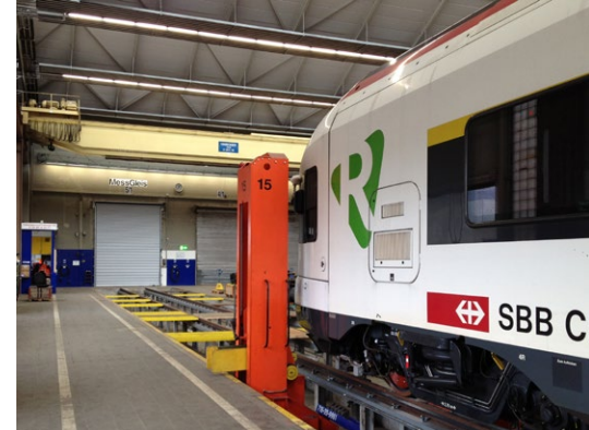
WILOC on elevated measuring track
